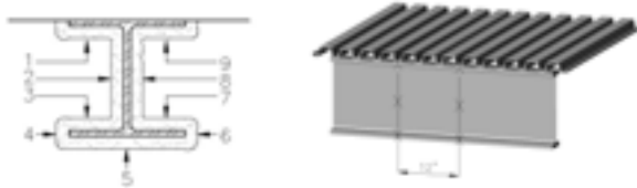
Fig. IX.2 SFRM Thickness Measurement Locations at Beams
